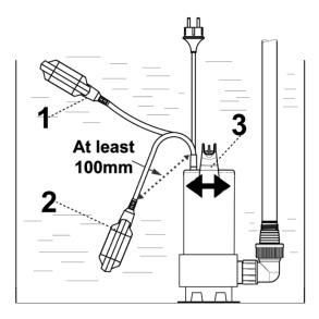
The pump will start pumping when the fluid has lifted the float switch fully (1).
